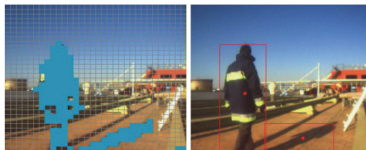
Fig. 6. Left) Object segmentation using motion. Right) Object segmentation using color.
